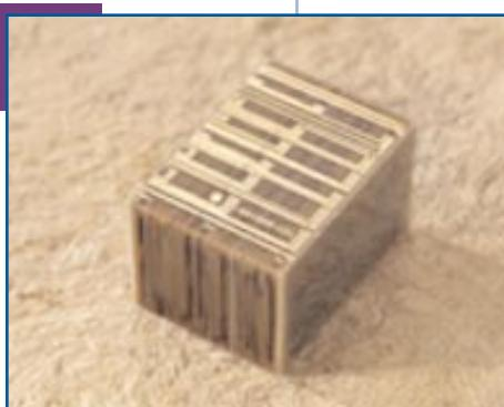
**Stacked, packed.** Chip-stacking technology facilitates extreme miniaturization of superconducting electronics, potentially enabling them to eliminate bottlenecks currently plaguing Internet and telecommunications traffic. Using this technology, Irvine Sensors is packaging SuperRouter™ switch electronics into a space comparable to the size of a fiber-optics cable.
